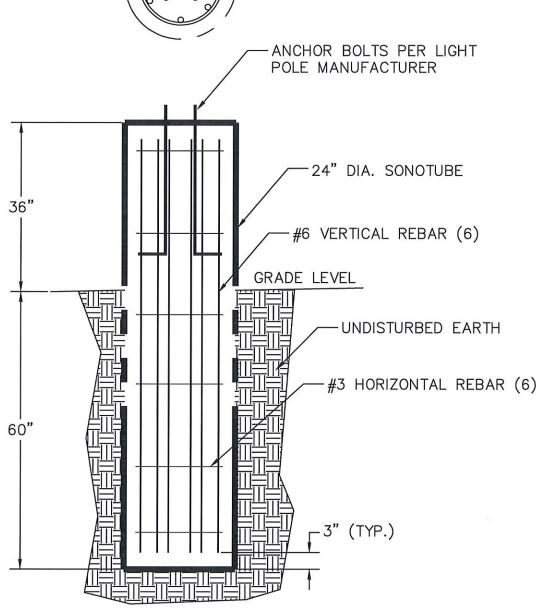
CONDUIT PER ELECTRICAL DESIGN CONCRETE SHALL BE 4000 PSI MIN.
