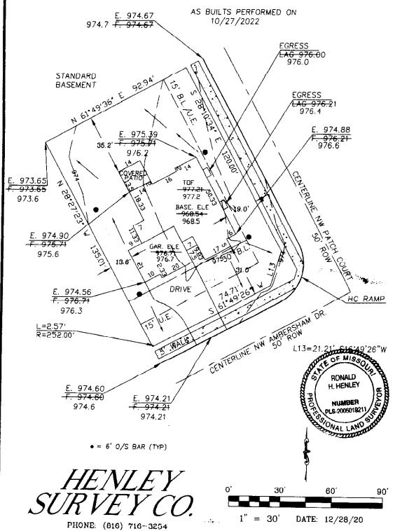
This plot plan was prepared for use before and during foundation construction only. House staked as shown on plot plan. Contractor to check and verify house dimensions and elevations at job site. We are not responsible for unknown or platted easements of any kind unless we are furnished the description of said easements before the field work is performed. NOTE. Cuts shown between for excession as a guide only. Final decision as to cuts and foundation height are to be made by builder on job site.
