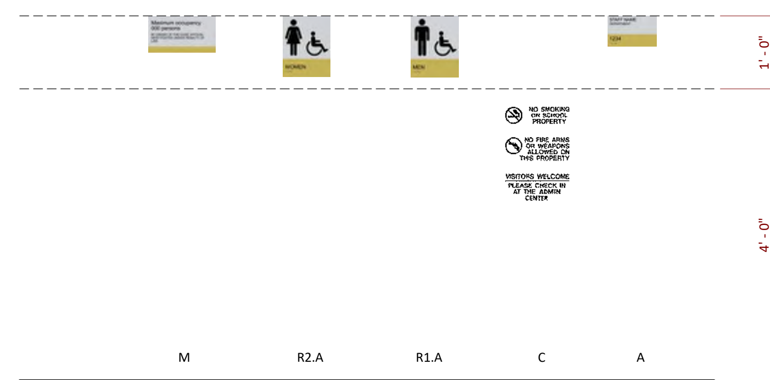
Typical Signage Mounting Heights A3
