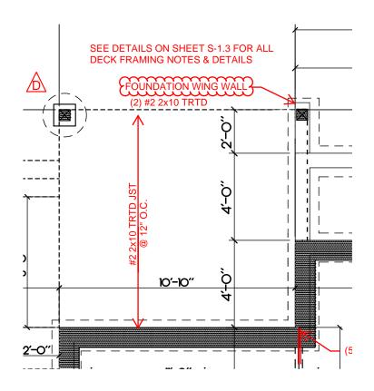
ALTERNATE POST BEARING AT REAR DECK
