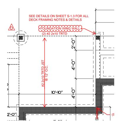
ALTERNATE POST BEARING AT REAR DECK
