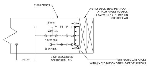
\* ALL LEDGERLOK SPACINGS NOT SHOWN SHALL BE CONSTRUCTED ACCORDING TO IRC 2018 SECTION R507.
