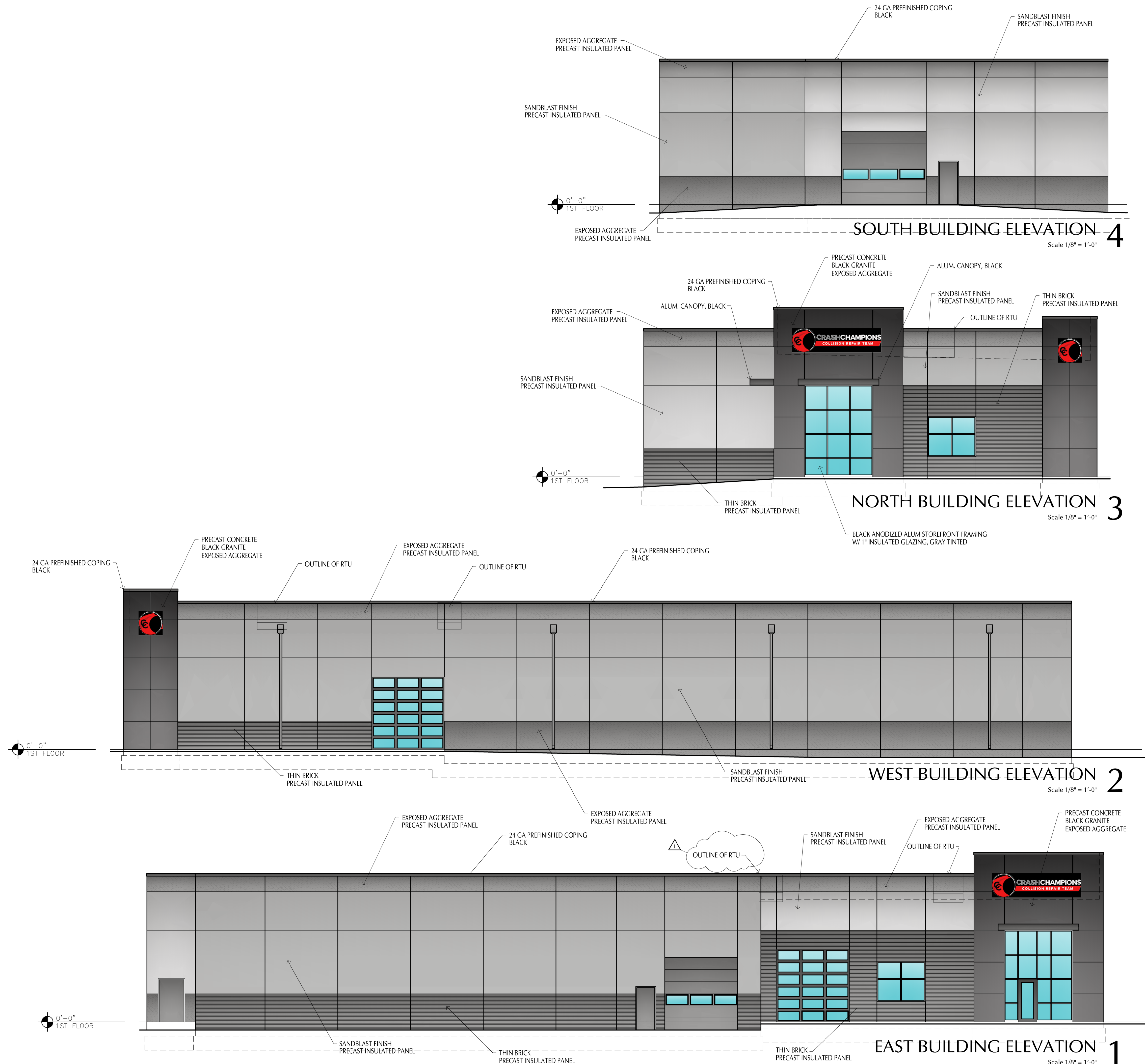
EXPOSED AGGREGATE OMEGA CONCRETE PRECAST INSULATED WALL PANEL COLOR: BLACK GRANITE
