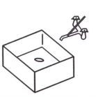
JANITOR SINK - WILLIAMS MODEL MTB-24"x24" FLOOR MOUNTED BASIN W/AMERICAN STANDARD 8341.075 FAUCET WITH VACUUM BREAKER. **INCLUDE VINYL BUMPER FOR EXPOSED SIDE &** PROVIDE P-TRAP FOR DRAIN. 1/2"H & CW, 3"WASTE, 2"VENT.
