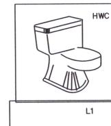
ROUND VITREOUS CHINA, ELONGATED FLOOR OUTLET, SIPHON JET ACTION, TANK TYPE TOILET W/WHITE, SOLID PLASTIC - KOHLER #KA716 OPEN FRONT SEAT LESS COVER. PROVIDE FLEXIBLE SUPPLY PIPE WITH WHEEL HANDLE STOP. 1/2", 4"WASTE. 2"VENT. HWC - HANDICAPPED WC GERBER, AQUA SAVER
