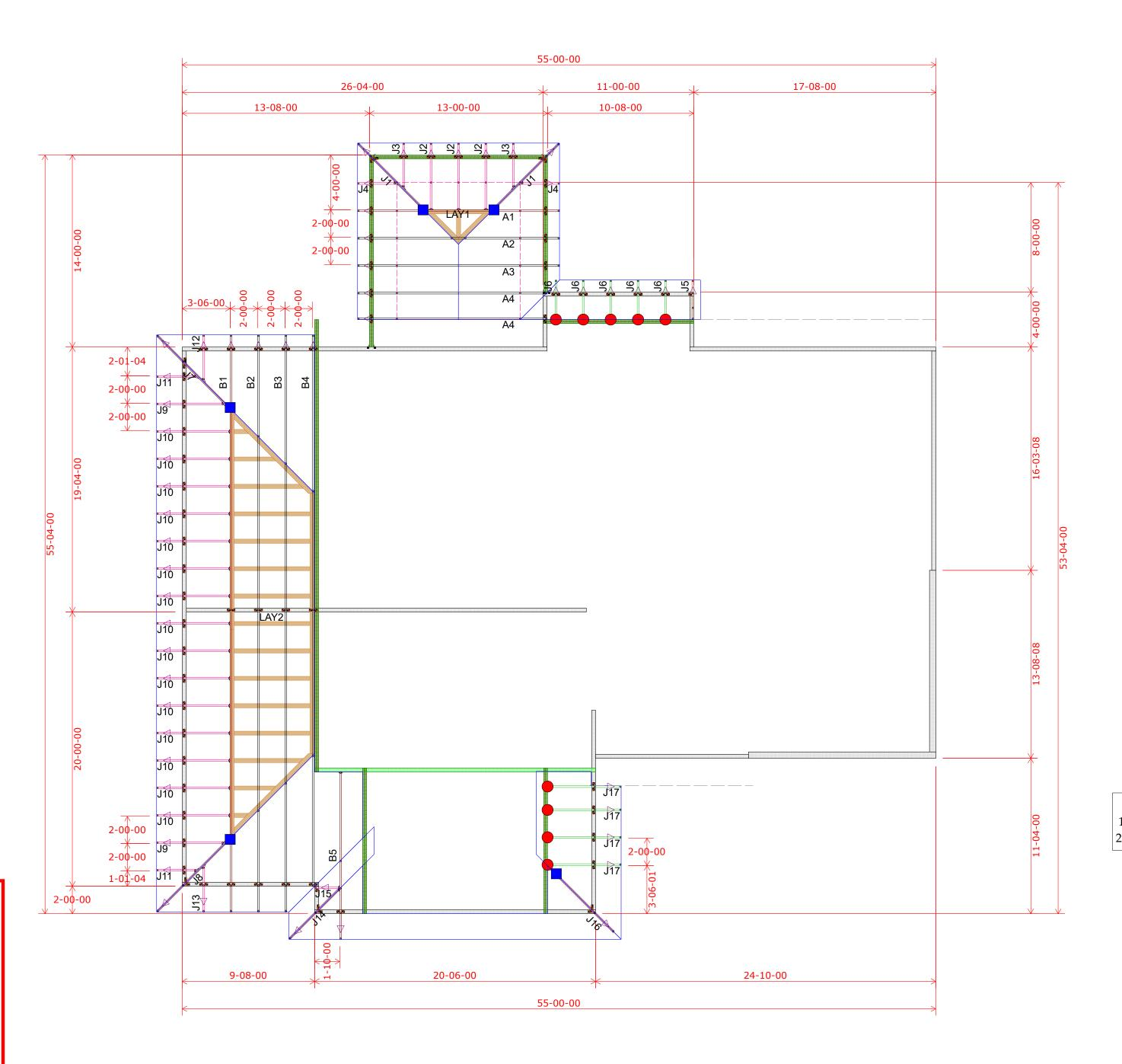
Roof Truss Layout Scale: 3/16" = 1'
