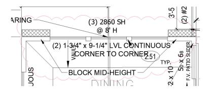
Inspection Comments: address top plate to top plate lap connection as required by code at front entry wall.
