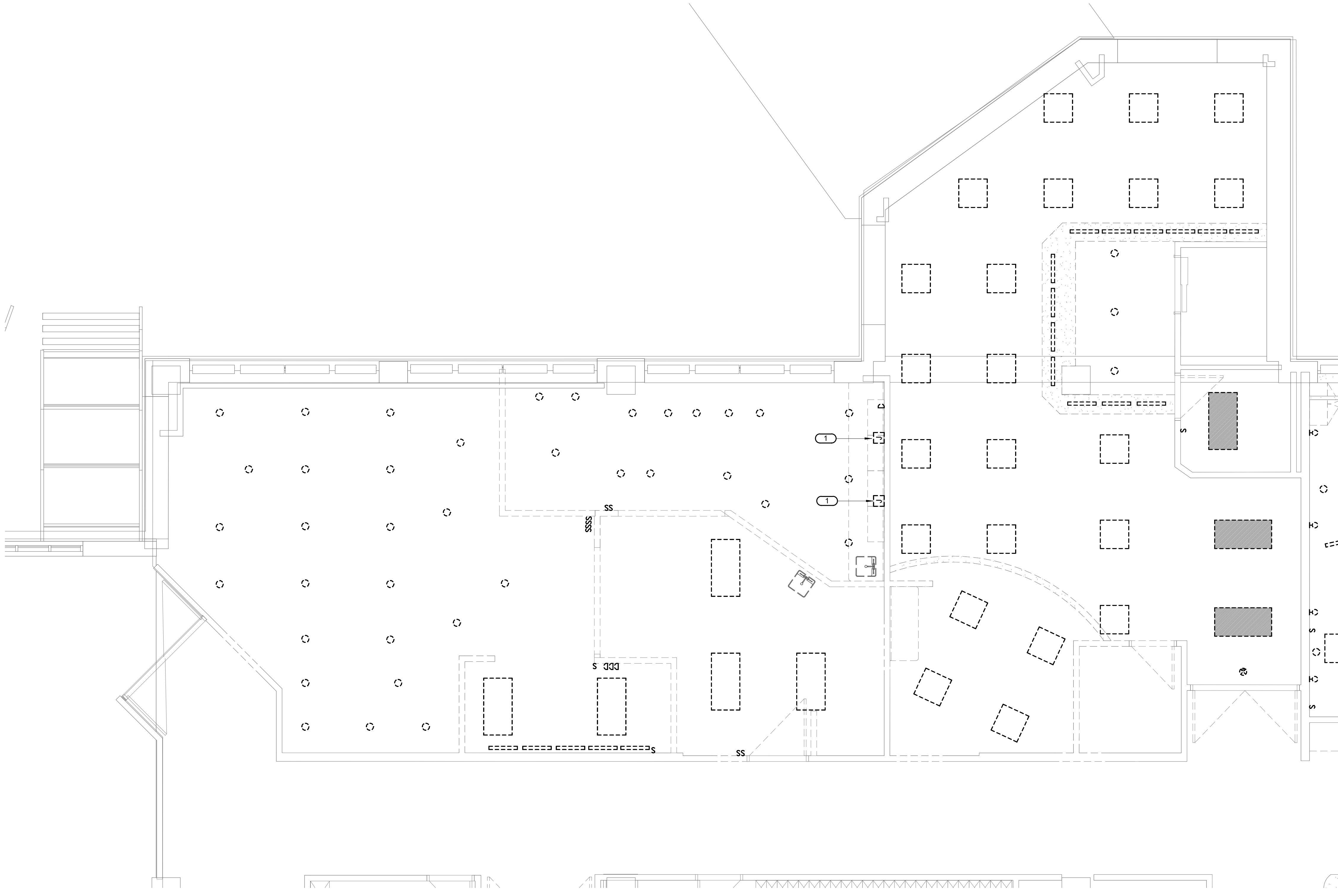
3 SECOND FLOOR DEMOLITION - LIGHTING - WELL BABY 1/4" = 1'-0"
