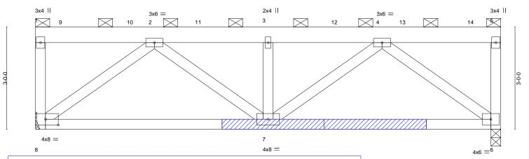
REPAIR: BOTTOM CHORD HAS 3/4" HOLE VERTICALLY THROUGH 1-1/2" FACE IN FRONT PLY ONLY 18" RIGHT OF JOINT 7
