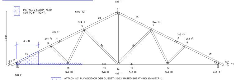
TO EACH FACE OF TRUSS WITH (0.131" X 2.5" MIN.) NAILS PER THE FOLLOWING NAIL SCHEDULE: 2 X 3'S - 2 ROWS, 2 X 4'S - 3 ROWS, 2 X 6'S AND LARGER - 4 ROWS: SPACED @ 4" O.C. NAILS TO BE DRIVEN FROM BOTH FACES. STAGGER SPACING FROM FRONT TO BACK FACE FOR A NET 2" O.C. SPACING IN EACH COVERED TRUSS MEMBER. USE 2" MEMBER END DISTANCE.
