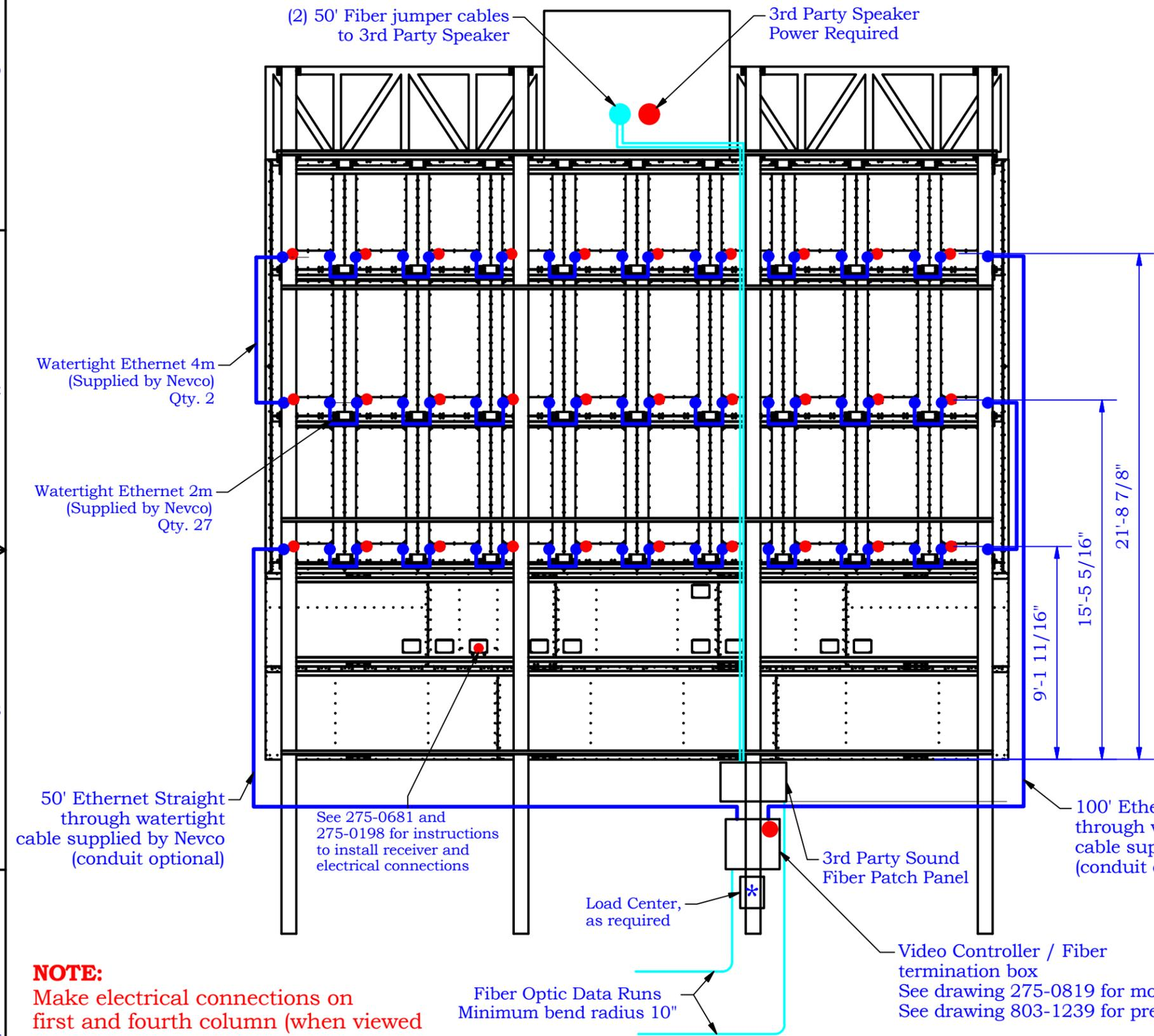
**Use high inrush current circuit breakers for video display.**
