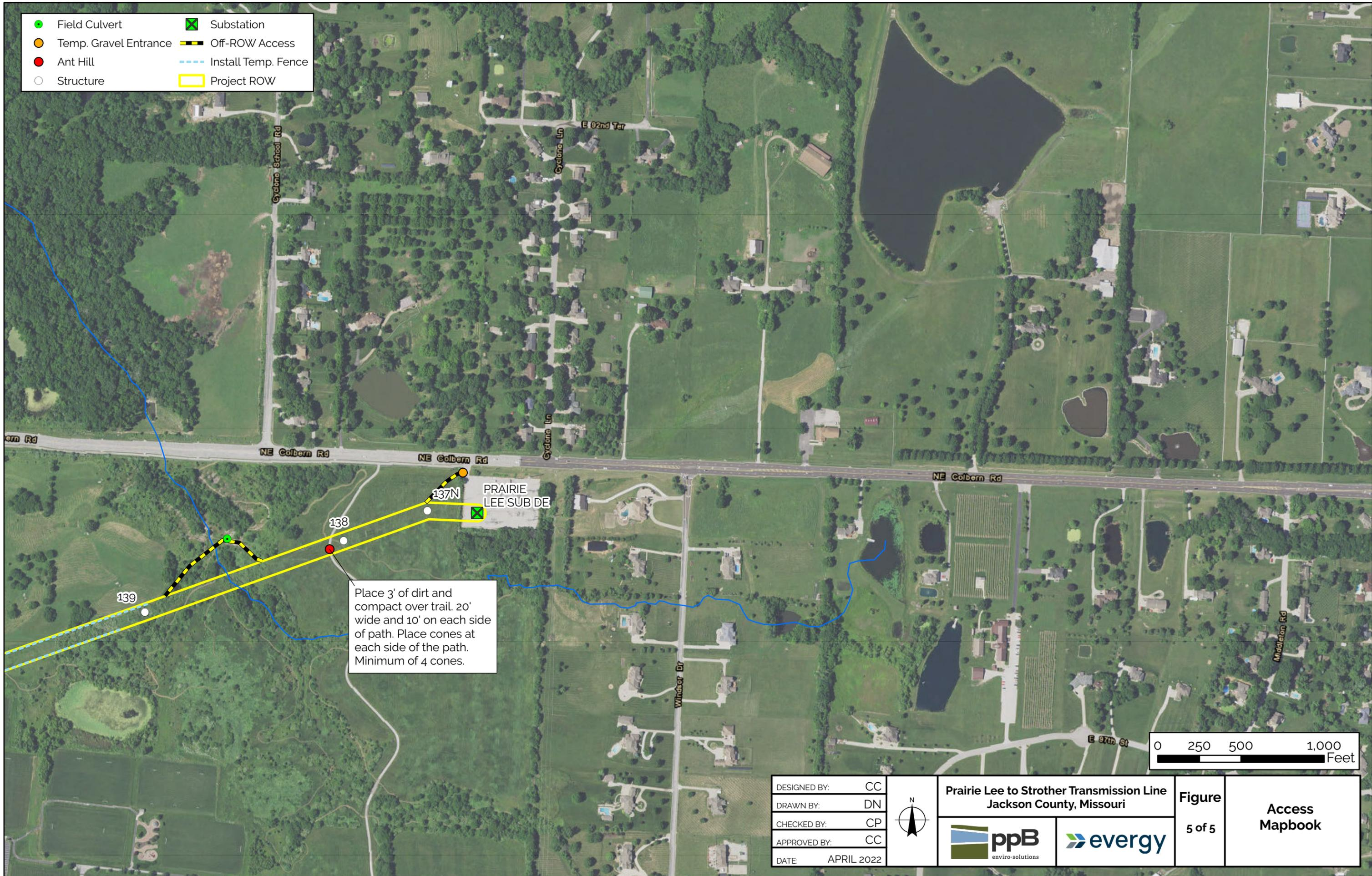
Place 3' of dirt and compact over trail. 20' wide and 10' on each side of path. Place cones at each side of the path. Minimum of 4 cones.
