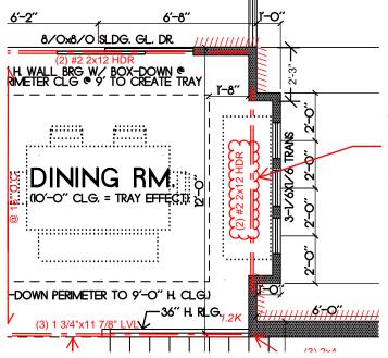
2X12 HEADER REQUIRED FOR LOAD TRANSFER CSPF OMITTED BASED ON SHEATHING CALCULATION REQ SHEET S-2.0
