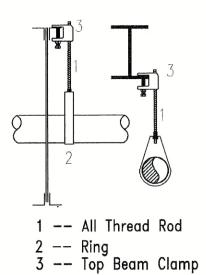
HANGER SPACING STEEL PIPE (EXCEPT THREADED LIGHTWALL) 1" -- 12 FT 1-1/4" -- 12 FT 1-1/2" -- 15 FT 2" -- 15 FT 2-1/2" -- 15 FT 3" -- 15 FT
