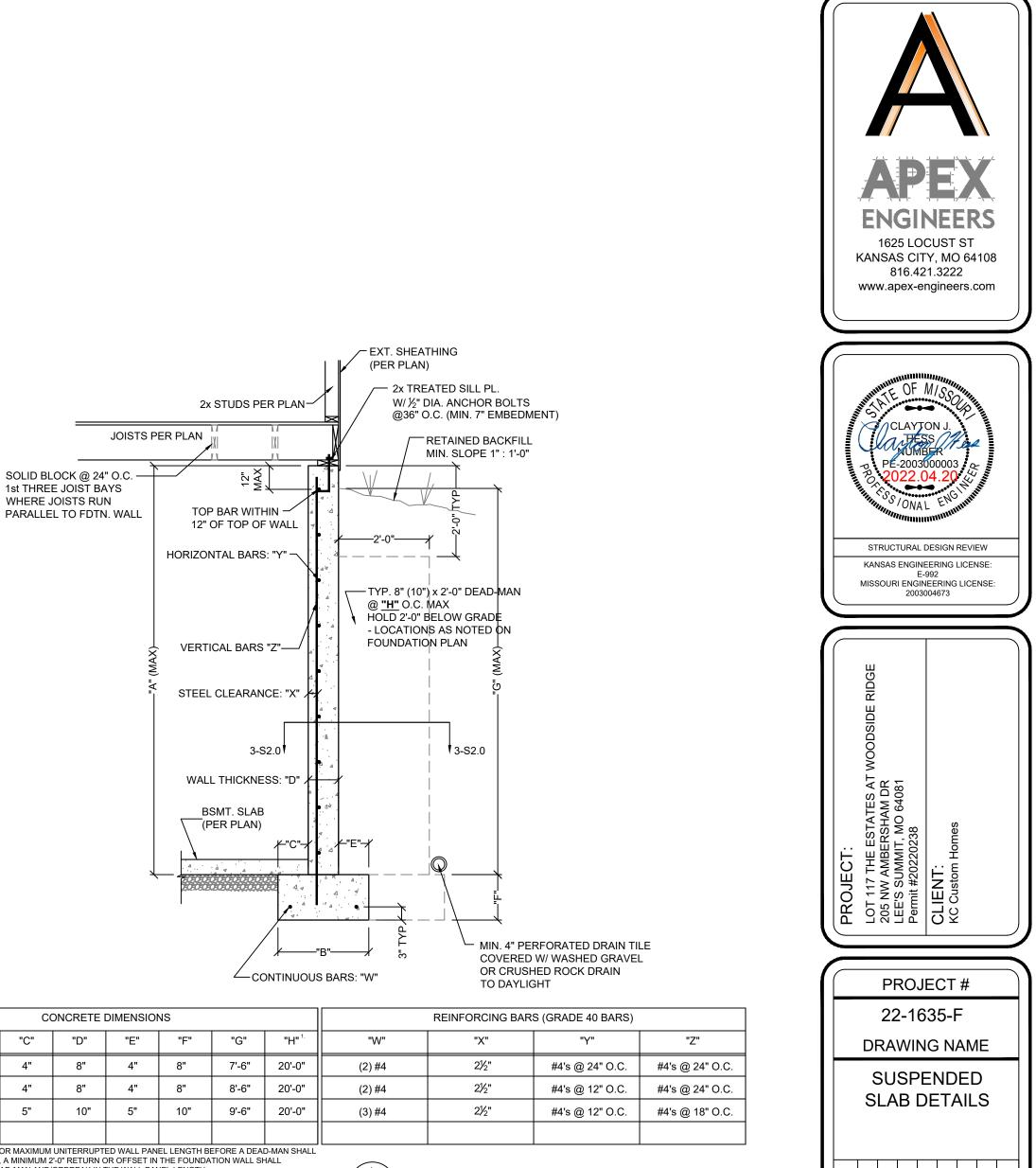
NAND/ORBREAK IN THE WALL PANEL LENGTH. L TO EXTEND TO WITHIN 8" OF TOP OF WALL. MINIMUM (1) #4 HORIZONTAL BAR WITHIN 12" OF TOP & BOTTOM OF WALL. 3. BURIED CONCRETE FOUNDATION WALLS UP TO 9'-0" TALL MAY BE 8" NOMINAL THICKNESS W/ #4 BARS
