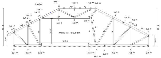
LUMBER MUST BE CUT CLEANLY AND ACCURATELY REMAINING LUMBER MUST BE UNDAMAGED AND UNDISTURBED.
