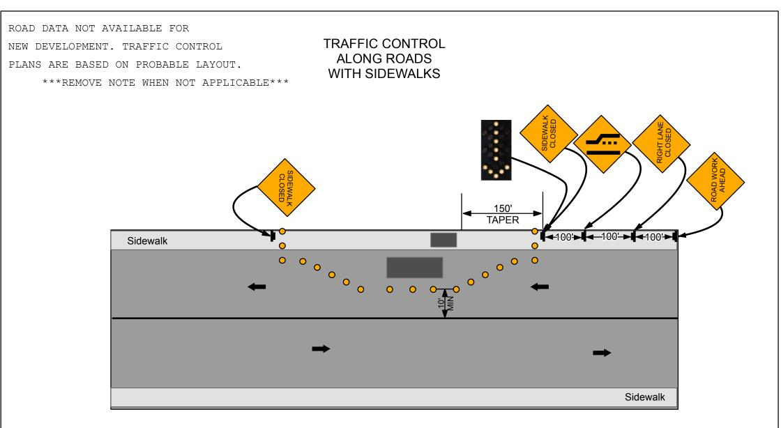
This plan is to be used on all 2 lane roads with sidewalks in this package. SW Blue Ribbon St, SW Chase Cir.
