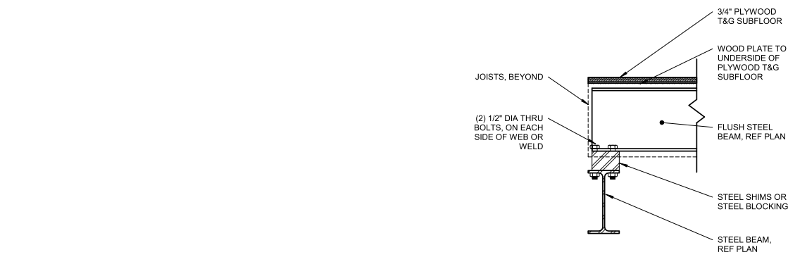
9 FLUSH STEEL BEAM TO STEEL BEAM S3.1 1 1/2" = 1'-0"
