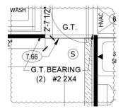
• Flex Room shall have (2) #2 2x4 Douglas Fir Larch studs at supports as shown in image below.
