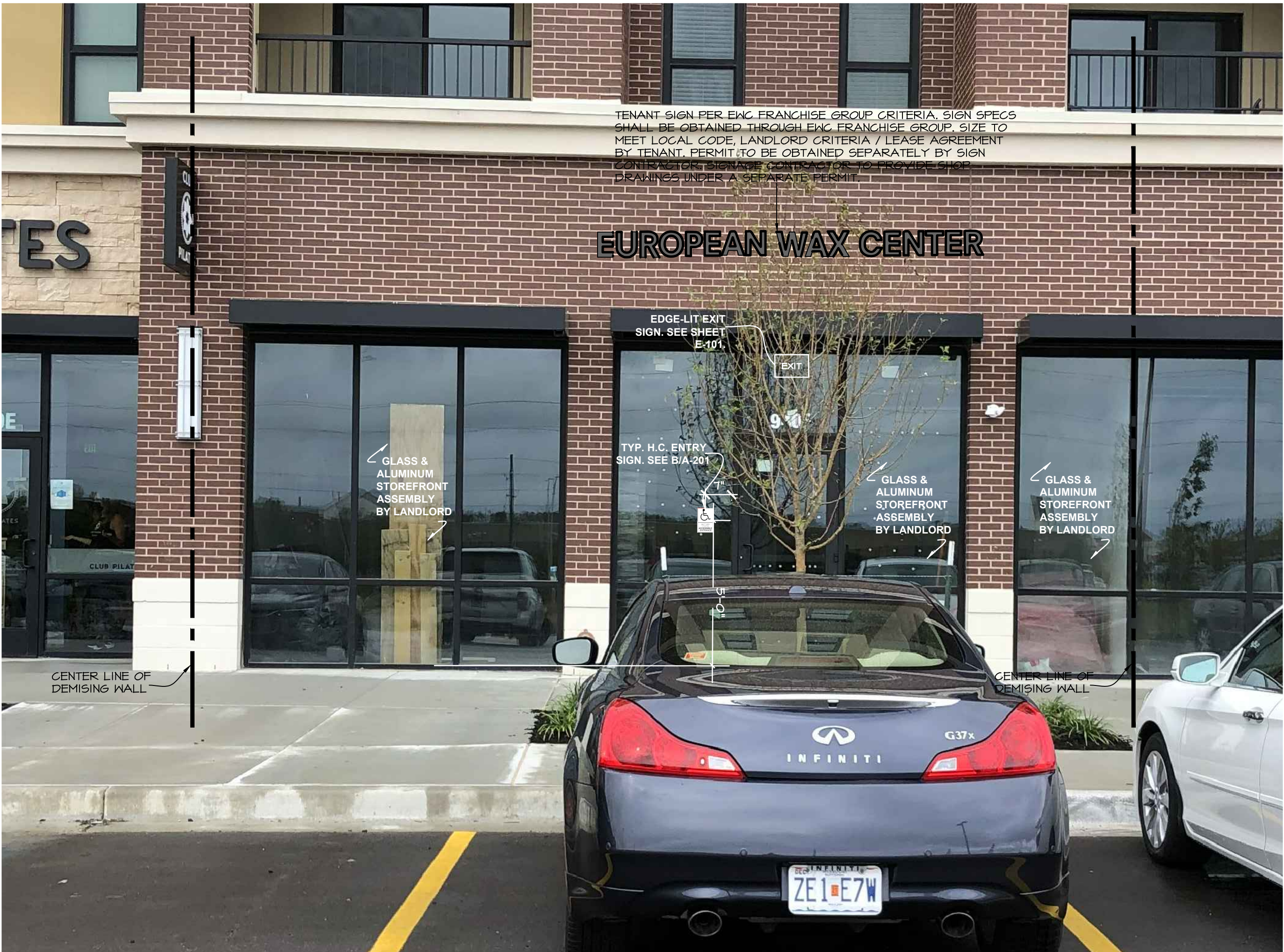
A STOREFRONT SIGNAGE ELEVATION
