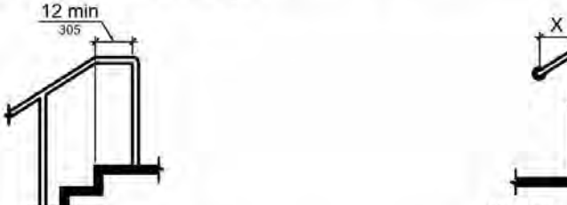
Figure 505.10.2 Top Handrail Extension at Stairs
