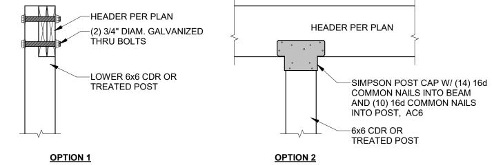
ROOF LEVEL INTERIOR BEAM TO COLUMN
