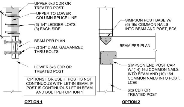
DECK LEVEL EXTERIOR BEAM TO COLUMN
