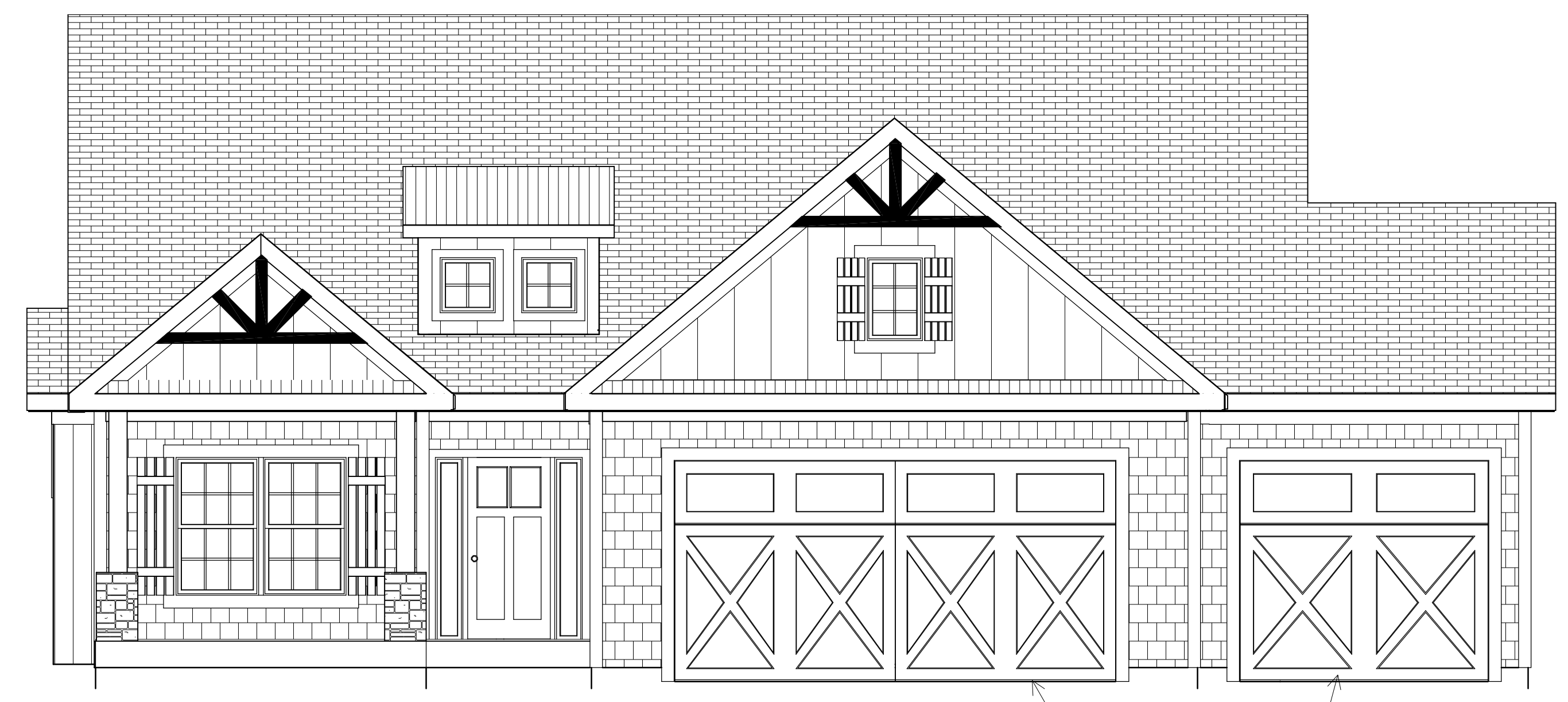
FRONT EL. SHAKE & BOARD AND BATT SIDING
