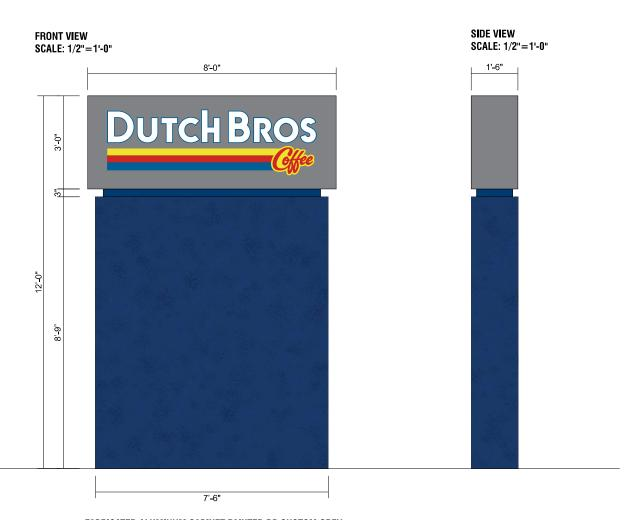
FABRICATED ALUMINUM CABINET PAINTED DB CUSTOM GREY. REVEAL PAINTED DB CUSTOM DARK BLUE. **BACKED-UP WHITE ACRYLIC LETTERS.** 1ST SURFACE 230-015 YELLOW, 230-33 RED, & 230-127 INTENSE BLUE PSV. WHITE LED ILLUMINATION. FABRICATED ALUMINUM SKIRT PAINTED DB CUSTOM DARK BLUE WITH MEDIUM TEXTURE COAT,
