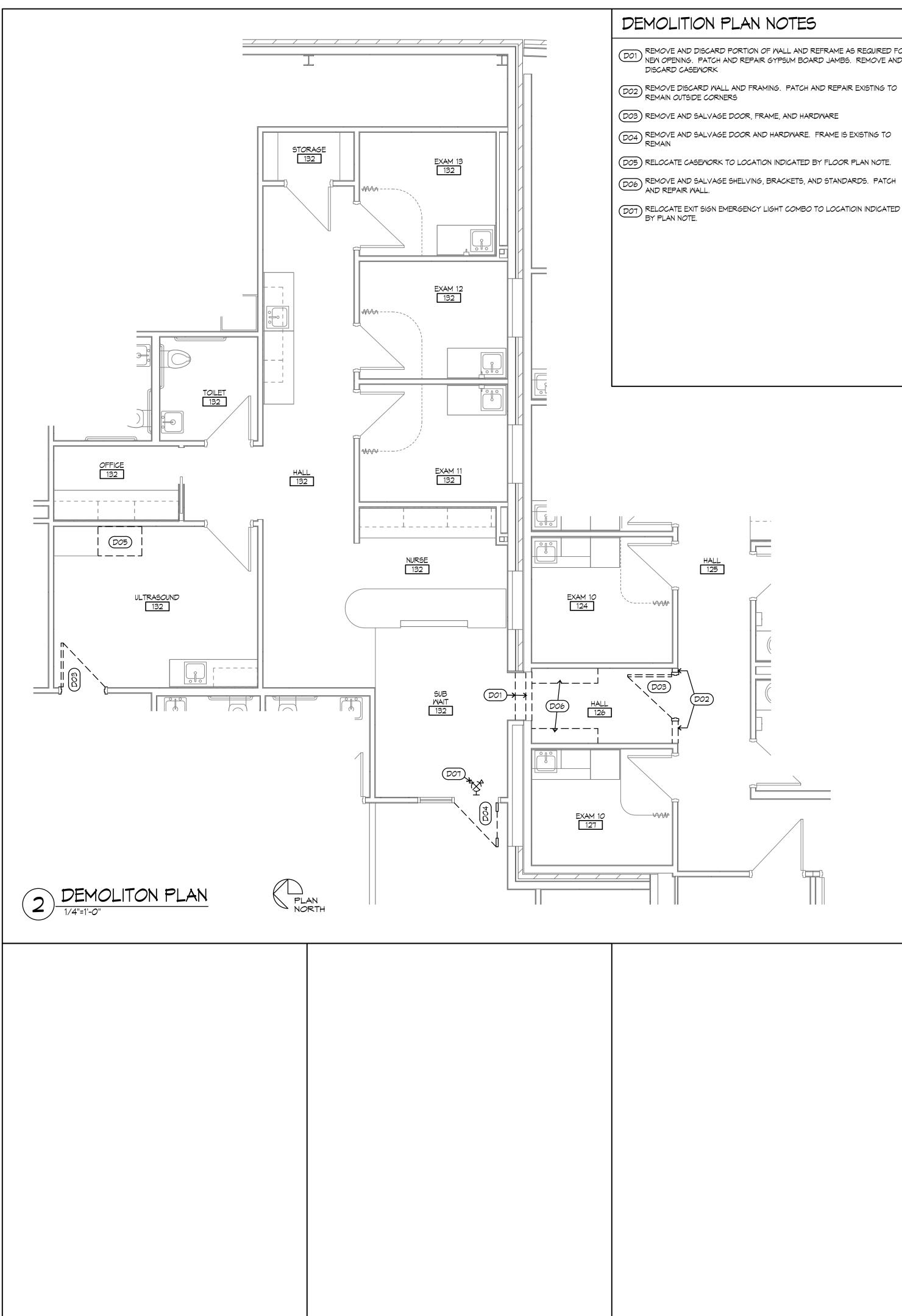
DO1 REMOVE AND DISCARD PORTION OF WALL AND REFRAME AS REQUIRED FOR NEW OPENING. PATCH AND REPAIR GYPSUM BOARD JAMBS. REMOVE AND
