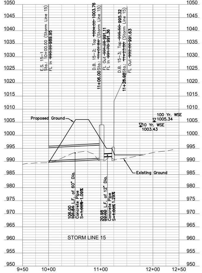
E.S. 15-1, Construct RCP End Section (60" RCP) w/ Concrete Toe Wall Sta.: 10+00.00 (Storm Line 15) N: 982,377.8600-982,381.7970 E: 2,813,817.9650-2,813,814.1540
