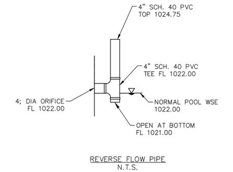
NOTE: CONTRACTOR SHALL FILL AND COMPACT TO 95% STANDARD DENSITY TO A POINT 18" MINIMUM ABOVE TOP OF PIPE PRIOR TO EXCAVATION FOR THE PIPE.
