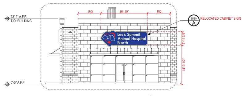
ENLARGED BUILDING ENTRY ELEVATION SCALE: 3/32" = 1'-0"
