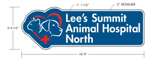
All noted dimensions are approximate and may be modified slightly during manufacturing to allow proper component usage.
