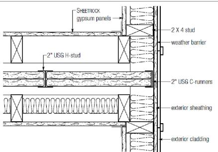
ONE LAYER 5/8" THICK GYPSUM BOARD (UL TYPE SCX™)
