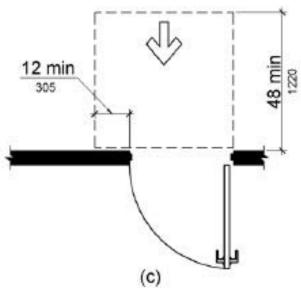
front approach, push side, door provided with both closer and latch
