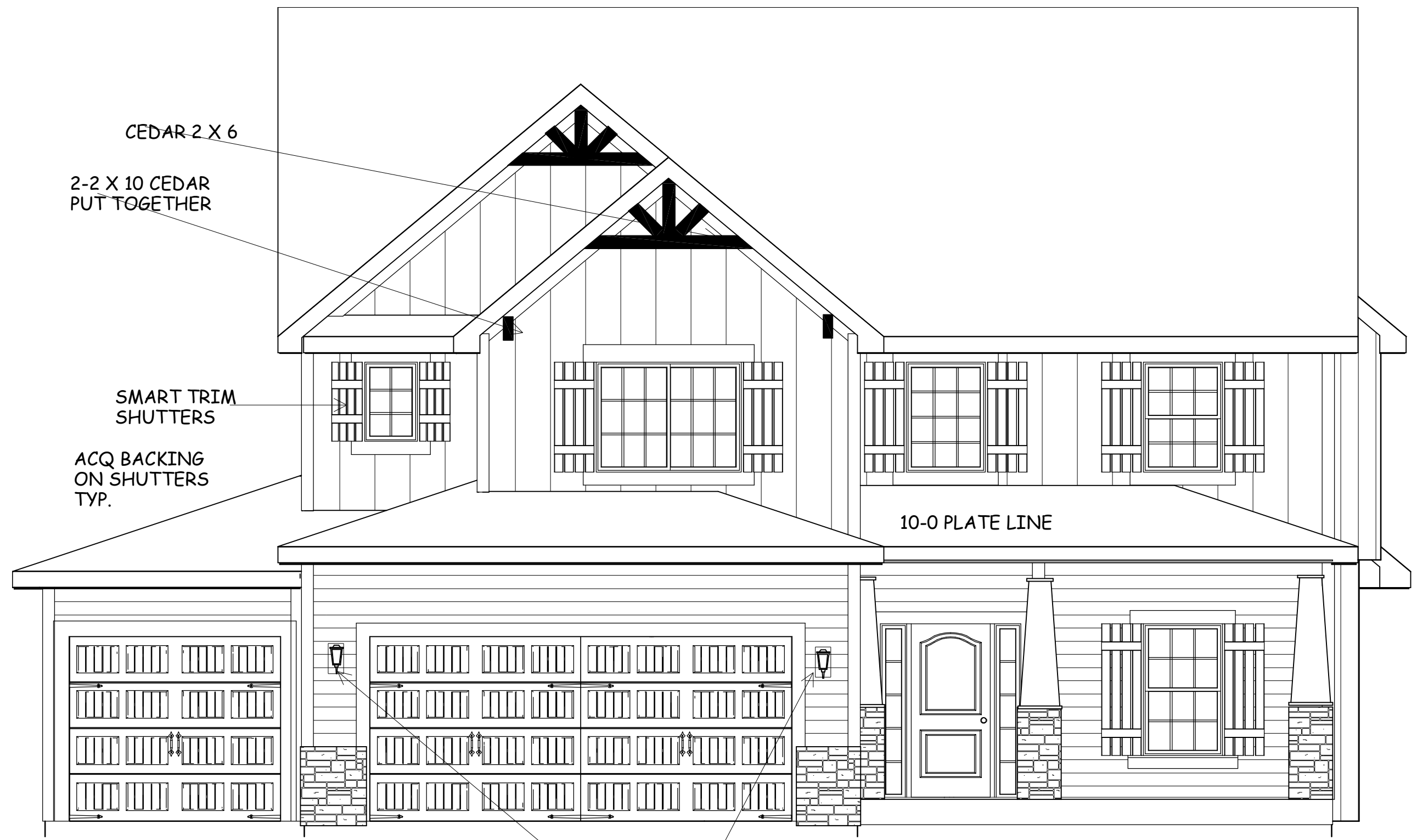
FRONT ELEVATION ELEVATION B
