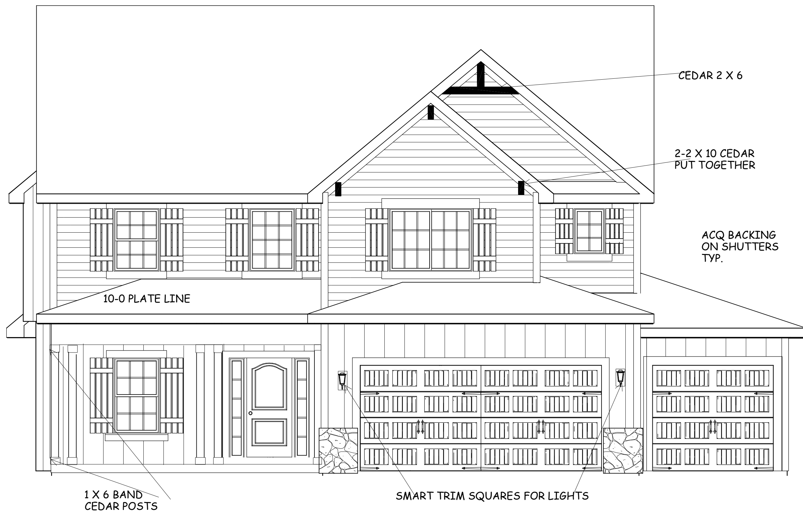
FRONT ELEVATION ELEVATION B
