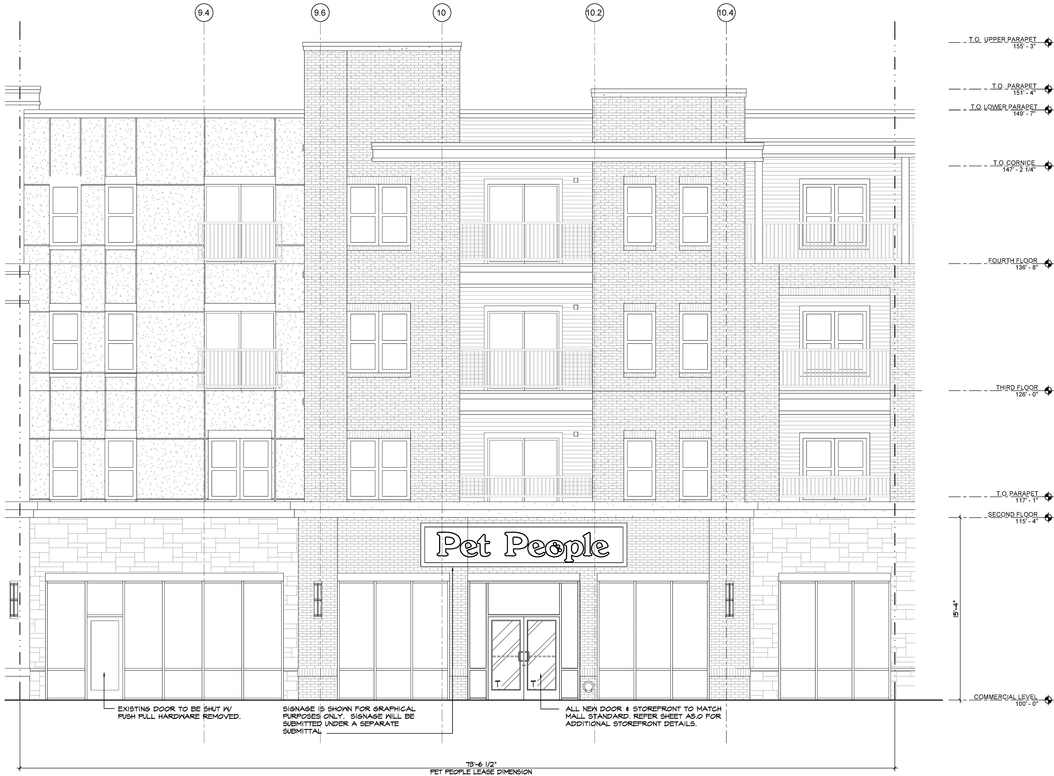
4 STOREFRONT EXTERIOR ELEVATION 1/4" = 1'-0"
