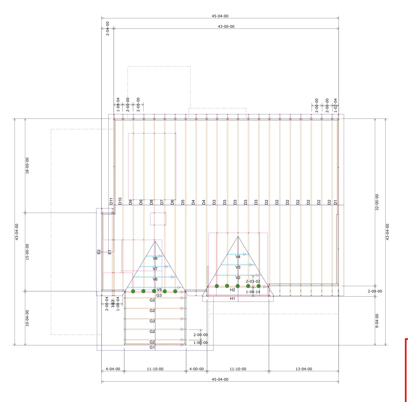
2nd Floor Truss Layout Scale: 3/16'' = 1'
