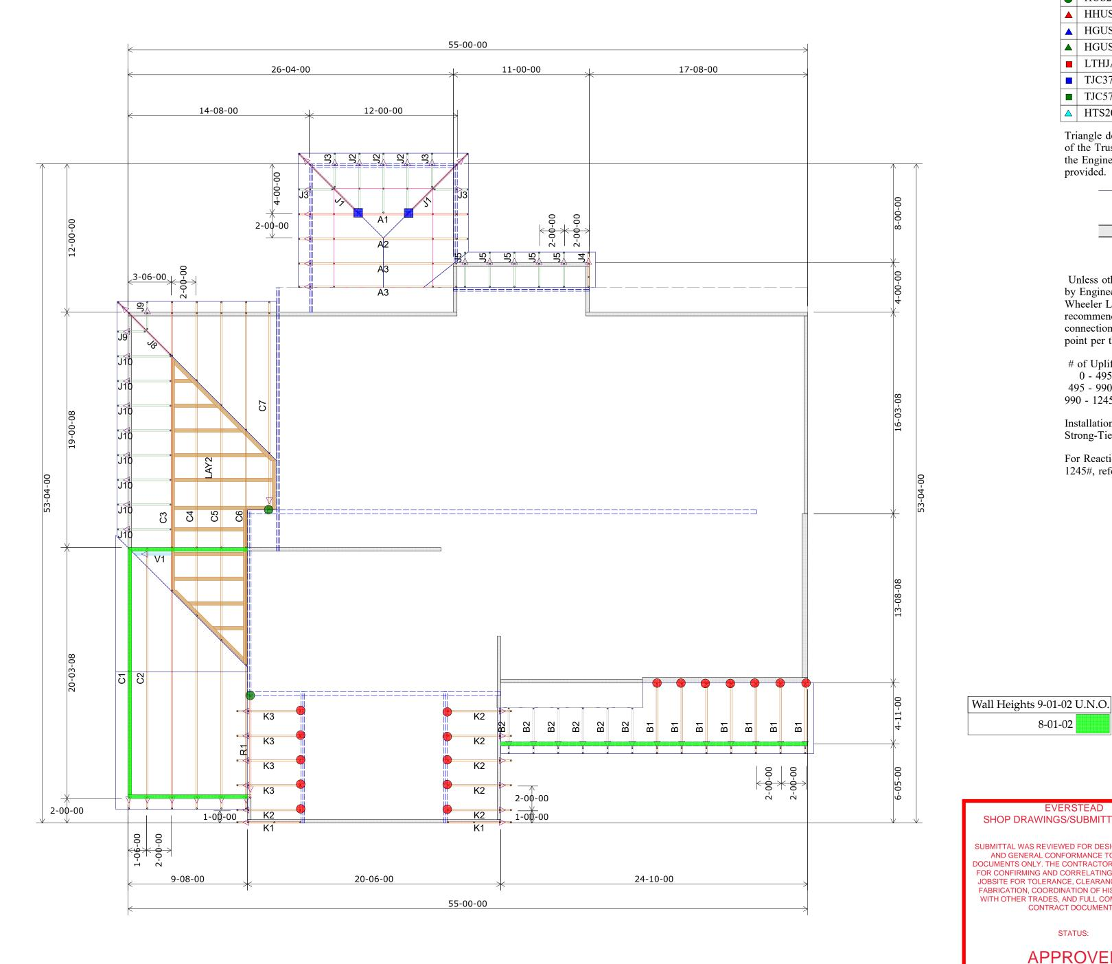
1st Floor Truss Layout Scale: 3/16'' = 1'
