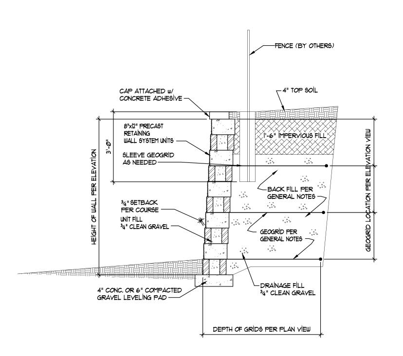
REINFORCED SOIL RETAINING WALL SECTION SCALE: 1/2" = 1'-0"
