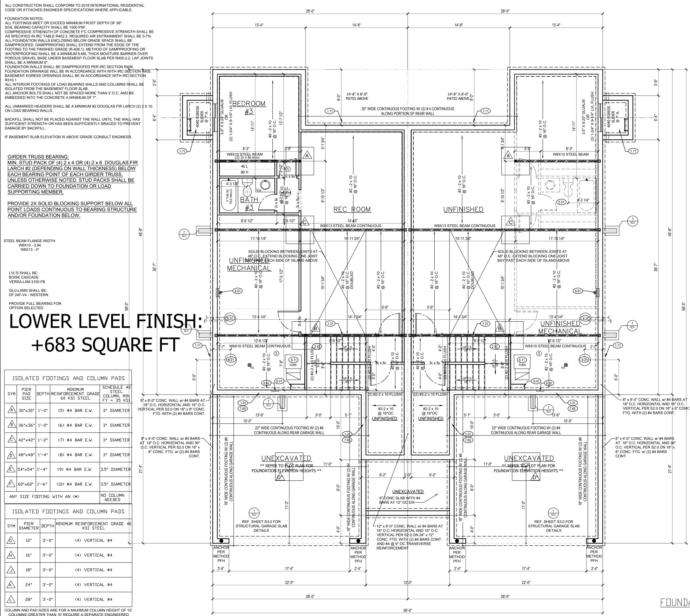
COLUMNS GREATER THAN 10' REQUIRE A SEPARATE ENGINEERED DESIGN. FOOTINGS A-F SPACING OF 6" O.C. WITH 3" CLEAR COVER.
