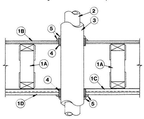
1. **Floor Assembly** — The fire rated wood truss or combination wood and steel truss Floor-Ceiling assembly shall be constructed of the materials and in the manner described in the individual L500-Series Designs in the UL Fire Resistance Directory and shall include the following construction features:
