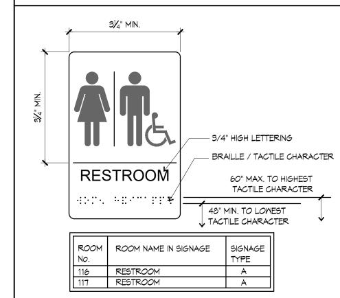
NOTE: ALL SIGNAGE TO MEET ICC/ANSI A117.1-2003 TACTILE CHARACTERS SHALL BE 48 INCHES (1220 MM) MINIMUM ABOVE THE FLOOR, MEASURED TO THE BASELINE OF THE LOWEST TACTILE CHARACTER AND 60 INCHES (1525 MM) MAXIMUM ABOVE THE FLOOR, MEASURED TO THE BASELINE OF THE HIGHEST TACTILE CHARACTER
