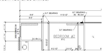
• It is structurally acceptable to install (3) Douglas Fir Larch #2 2x4's below stud pack above at stair support with footing "A" as shown in image below.
