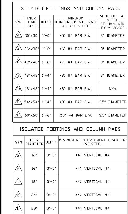
COLUMN AND PAD SIZES ARE FOR A MAXIMUM COLUMN HEIGHT OF 10'.
