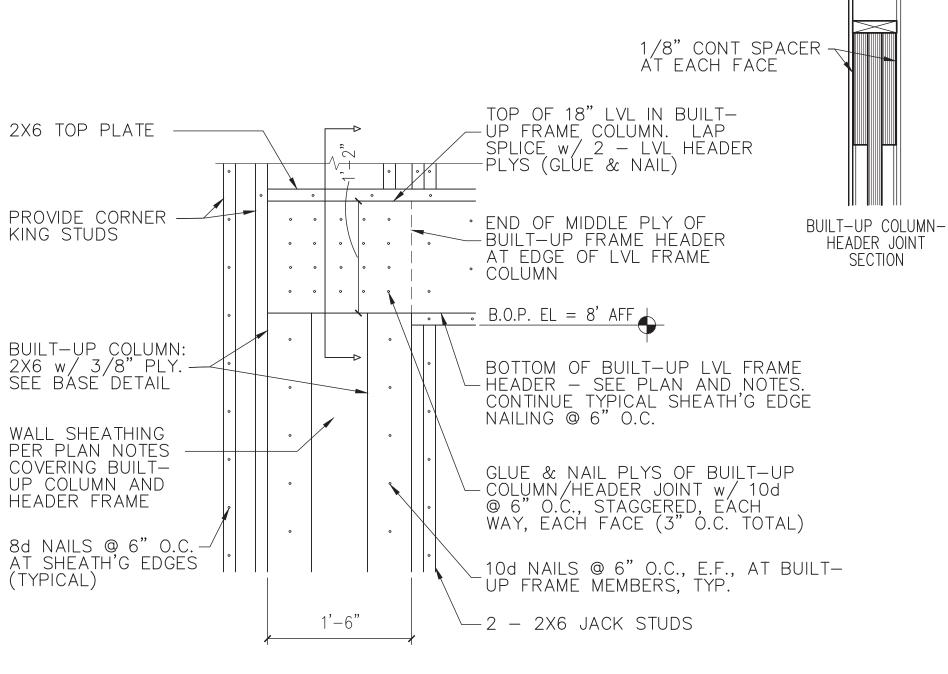
LVL SHEAR FRAME HEADER-COLUMN JOINT DETAIL ∖S201 SCALE = NONE
