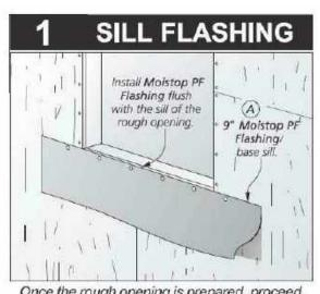
Once the rough opening is prepared, proceed by attaching Moistop PF Flashing (A) flush along the bottom of the rough opening. Be sure not to fasten the lower edge of the flashing so that Jumbo Tex®, Fortify® or WeatherSmart™ may be slipped up underneath the flashing in a weather-board fashion, extend the flashing beyond the jamb flashing to be applied later.
