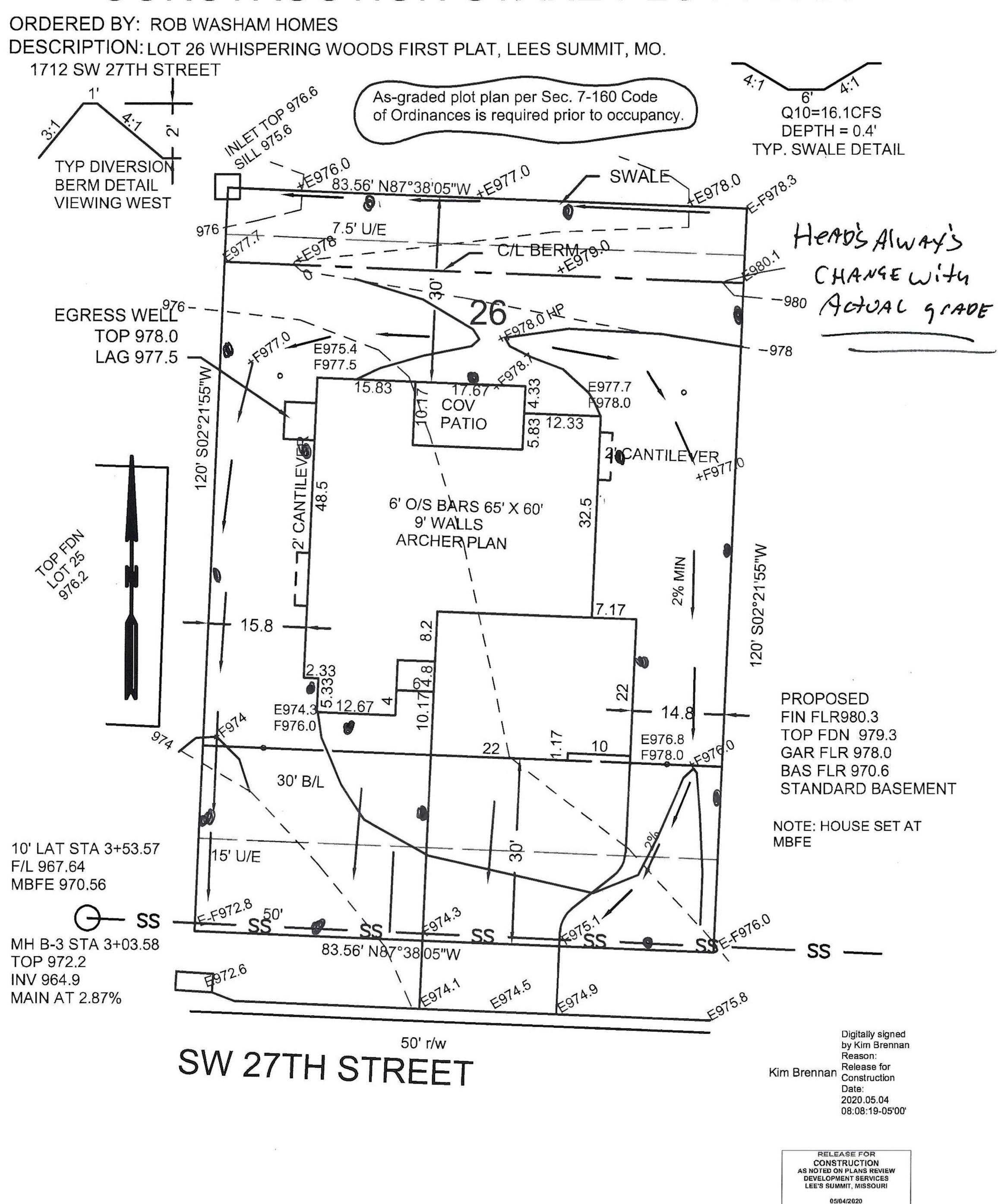
This plot plan is not an "as-built" survey as the house was staked prior to being built and cannot be used in place of a "Surveyors Real Property Report". This plot plan was prepared for use before and during foundation construction only and should not be used to establish property lines for fences or other structures. House staked as shown on this plot plan. House dimensions may have been
