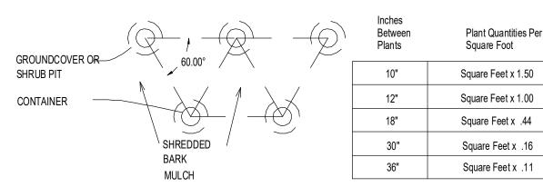
NOTES: 1. SPACING FOR GROUNDCOVERS, SHRUBS, AND PERENNIALS NOTED ON PLANS. 2. TILL SOIL IN BED TO A 12" MINIMUM DEPTH AND THOROUGHLY MIX IN SOIL AMENITIES AS NOTED ON PLANS.
