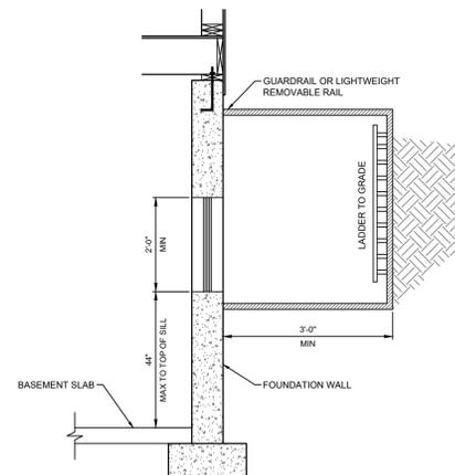
3 S3.0 TYPICAL EGRESS WINDOW SECTION DETAIL N.T.S.
