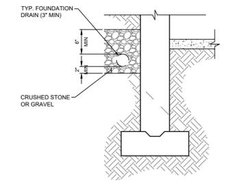
**1** FOUNDATION DRAIN DETAIL & RAISED SLAB
