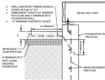
8 S3.0 ALTERNATE SLAB AT WALL N.T.S.
