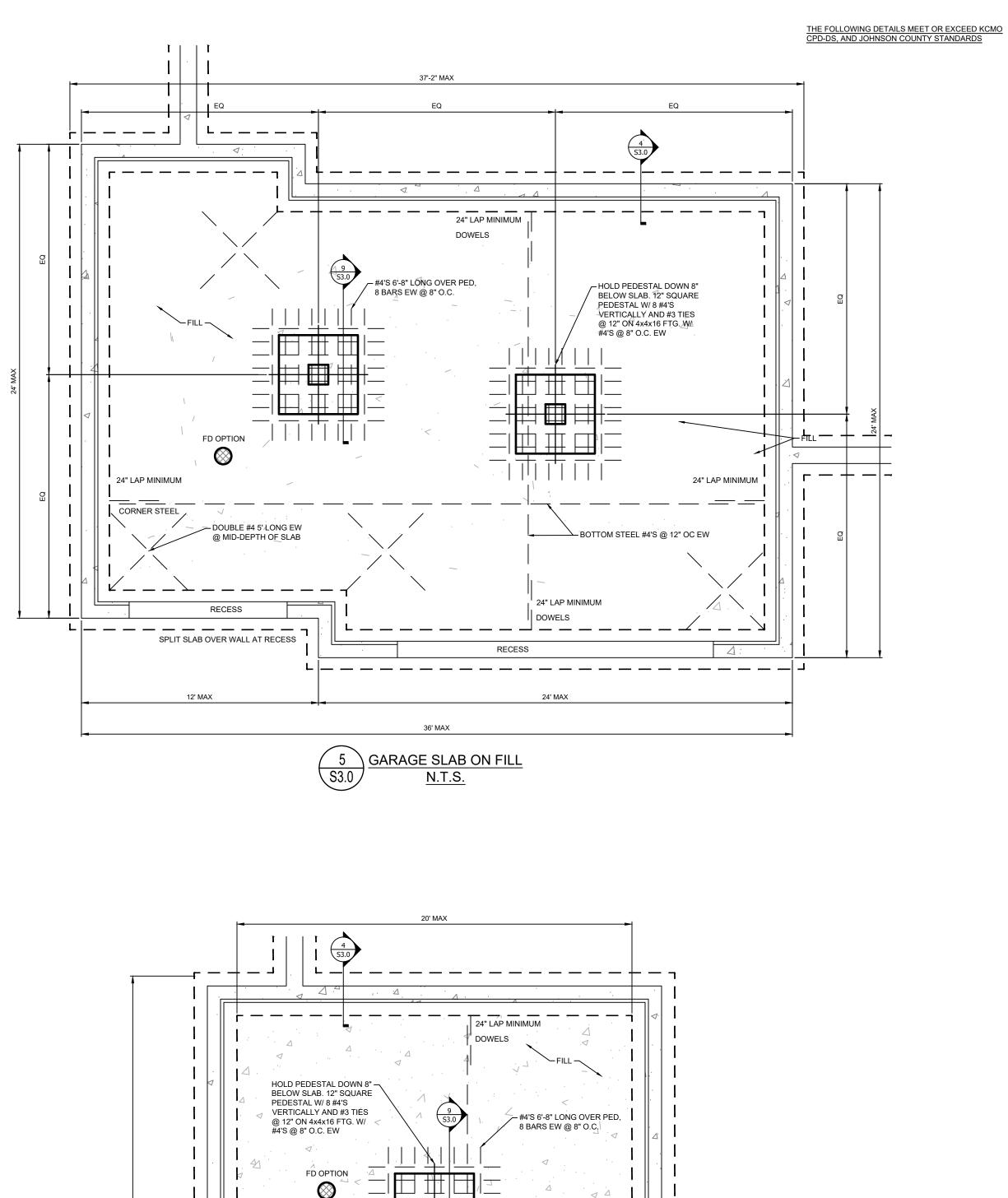
$\bigotimes$ 24" LAP MINIMUM DOWELS DOWELS ∽ FII I – BOTTOM STEEL #4'S @ 12" OC CORNER STEEL - DOUBLE #4 5' LONG EW @ MID-DEPTH OF SLAB 24" LAP MINIMUM DOWELS RECESS \_ \_ \_ \_ \_ \_ \_ \_ \_ \_ \_ \_ \_ \_ \_ \_ \_ SPLIT SLAB OVER WALL AT RECESS 12' MAX 24' MAX GARAGE SLAB ON FILL 1 <u>N.T.S.</u> S3.0
