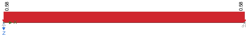
Roof Live - Loading (kips/ft)
