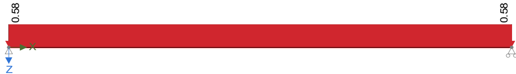
Roof Live - Loading (kips/ft)
