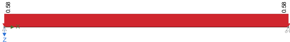
Roof Live - Loading (kips/ft)
