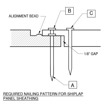
NAILING WITH SPACING AS SPECIFIED PER PLAN. FOR EXAMPLE, IF REQUIRED SPACING IS 4" O.C., BOTTOM LAP SHALL FIRST BE NAILED AT 4" O.C. (NAIL "A"), THEN OVERLAP SHALL BE NAILED @ 4" O.C. STAGGERED BETWEEN BOTTOM LAP NAILING (NAIL "B"), THEN FULL DEPTH SECTION OF OVERLAP PANEL SHALL BE NAILED @ 4" O.C. (NAIL "C")
