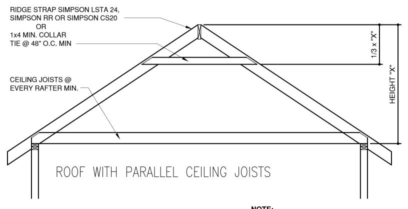
ROOF FRAMING DETAIL A-DTV-06100-04
