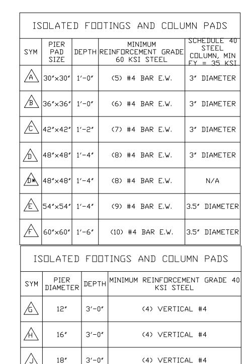
COLUMN AND PAD SIZES ARE FOR A MAXIMUM COLUMN HEIGHT OF 10'.
